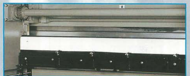
• Bottom Die/Table Hydraulic Support, ensure bent workpiece in straight alignment.
